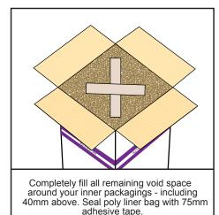
Close top flaps of box and seal closed with 75mm adhesive tape in 'U' shape
