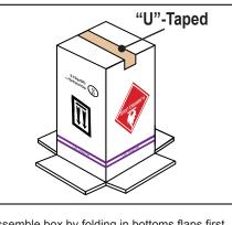
Assemble box by folding in bottoms flaps first. Seal flaps with 75mm adhesive tape in a 'U' shape
