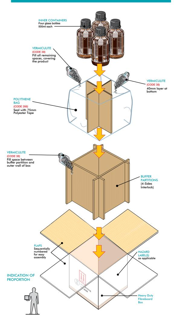
DE: 1007 GB/6539 FOR GROUPS: | || ||| ХΥ Ζ 4G/X7/S/\*\* GB/6539 UP TO A **GROSS PACKAGE** 7<sub>kg</sub> WEIGHT OF: UP TO INNER 4 **CONTAINERS External Dimensions:** 264 x 264 x 314mm **Internal Dimensions:** Four Cells - 100mm Square 100 x 100 x 230mm NOTES:
